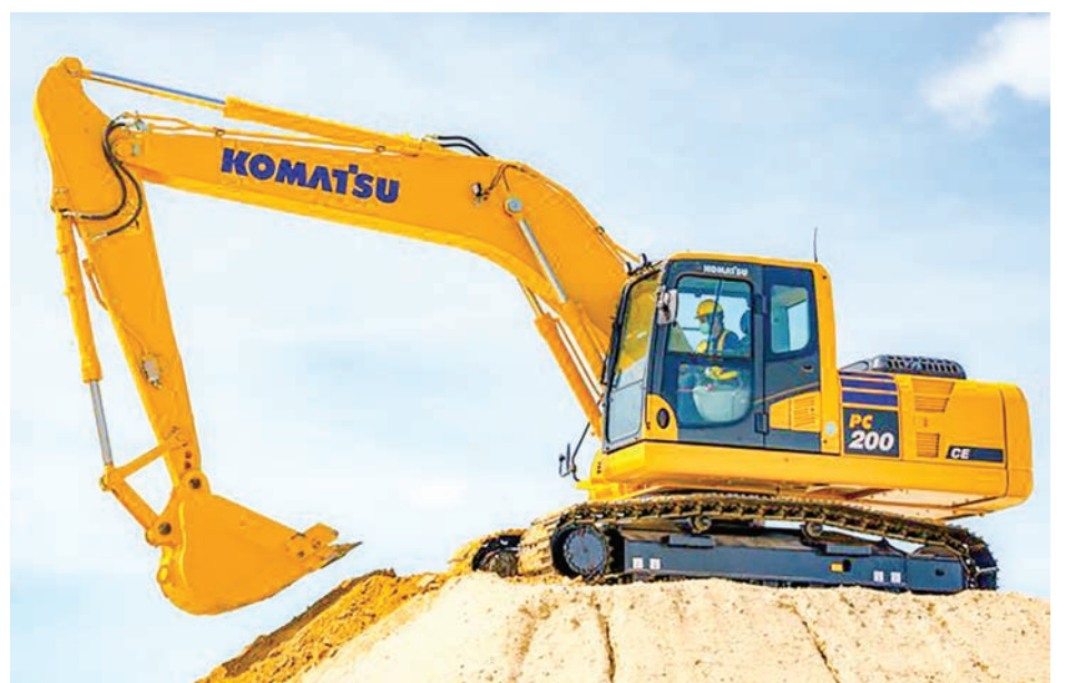
Photo shows Komatsu Ltd.'s 20-tonne PC200-10M0 hydraulic excavator under the CE series for use in urban civil engineering. The Japanese construction machinery maker began selling the new model in Southeast Asia in July 2021. PHOTO: KYODO
