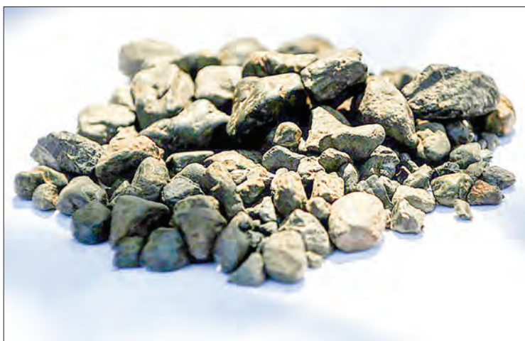
Coltan is a highly lucrative source of niobium and tantalum, which are used in electronics and high-performance alloys. PHOTO: AFP
