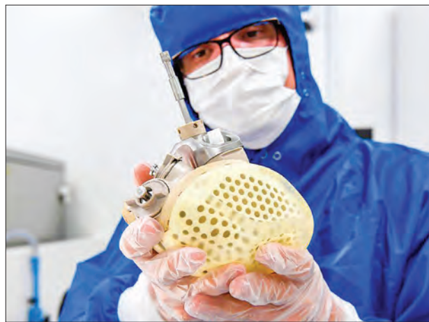
A Carmat employee shows an auto-regulating, bioprosthetic artificial heart. PHOTO: BERTRAND GUAY/AFP
