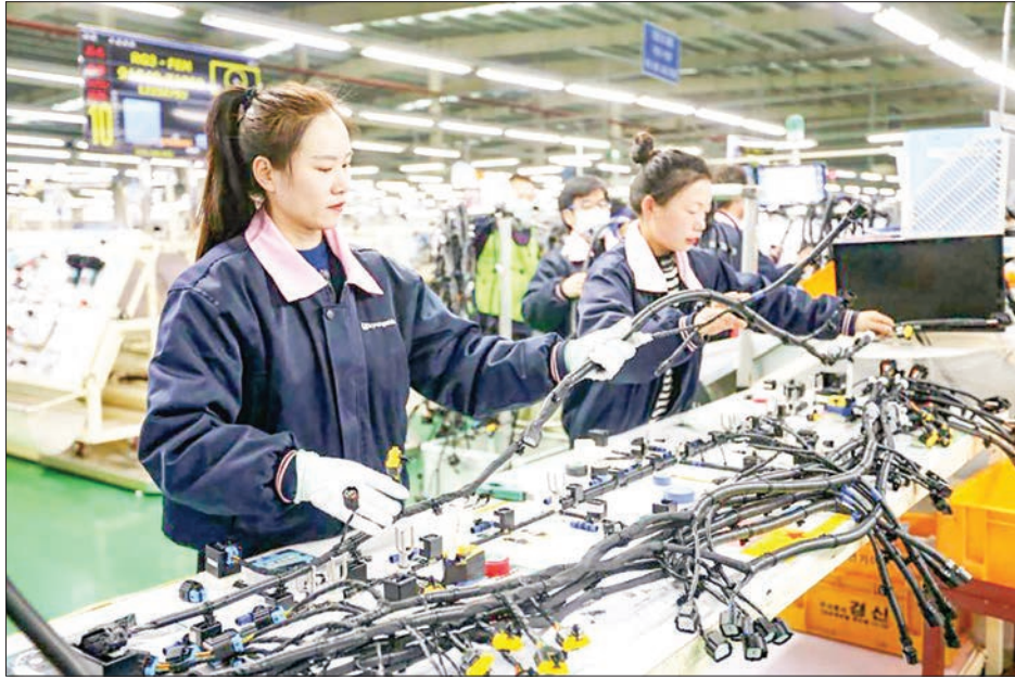
Employees at a car accessories factory in Huaibei, China. PHOTO: STR / AFP
