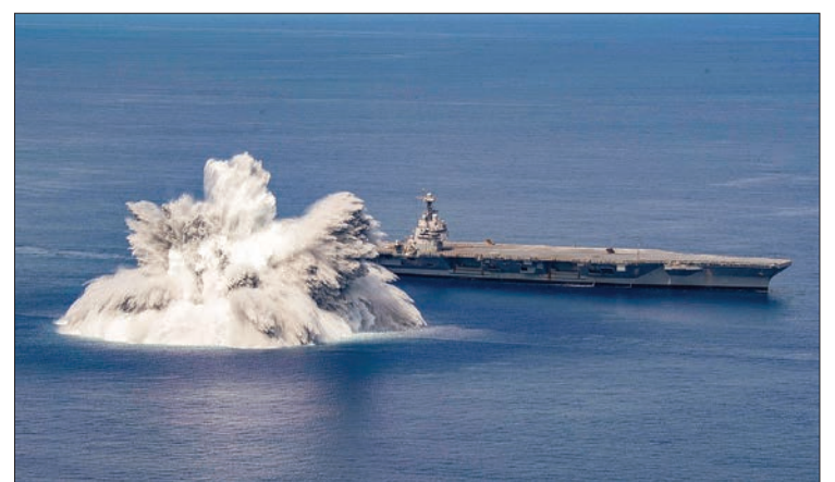
In this handout image courtesy of the US Navy the aircraft carrier USS Gerald R. Ford (CVN 78) completes the first scheduled explosive event of Full Ship Shock Trials while underway in the Atlantic Ocean, 18 June 2021. The US Navy has started carrying out what it calls 'Full Ship Shock Trials' by detonating powerful explosions to test whether its aircraft carriers are ready for war. PHOTO: AFP
