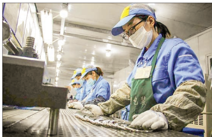
Workers checking aluminum pistons for vehicle engines on a production line at a machine manufacturing factory in Binzhou, in eastern China's Shandong province. PHOTO: AFP
