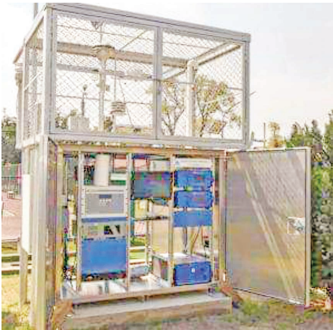
The photo shows a machine measuring air quality index.
