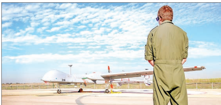
A soldier watches an Israeli IAI Heron TP drone on a tarmac. The IAI Heron TP is a multirole, advanced, long-range Medium Altitude Long Endurance, Unmanned Aerial System for strategic missions. PHOTO COURTESY IAI
