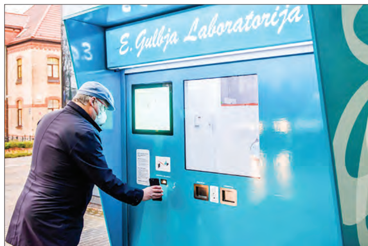
The automated centre hands out testing kits with a robot arm and then collects the samples. PHOTO: AFP
