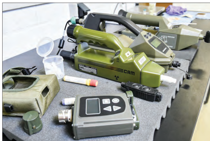
A picture shows a flame photometric detector and an ion mobility spectrometer at the OPCW (The Organization for the Prohibition of Chemical Weapons) headquarters in The Hague, The Netherlands, on April 20, 2017. PHOTO: AFP
