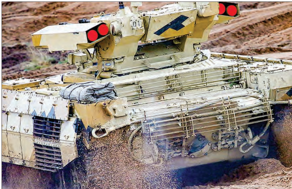
The vehicle is equipped with two 30mm-caliber 2A42 autocannons and a 7.62mm-caliber PKTM twin-mount machine gun. PHOTO: TASS
