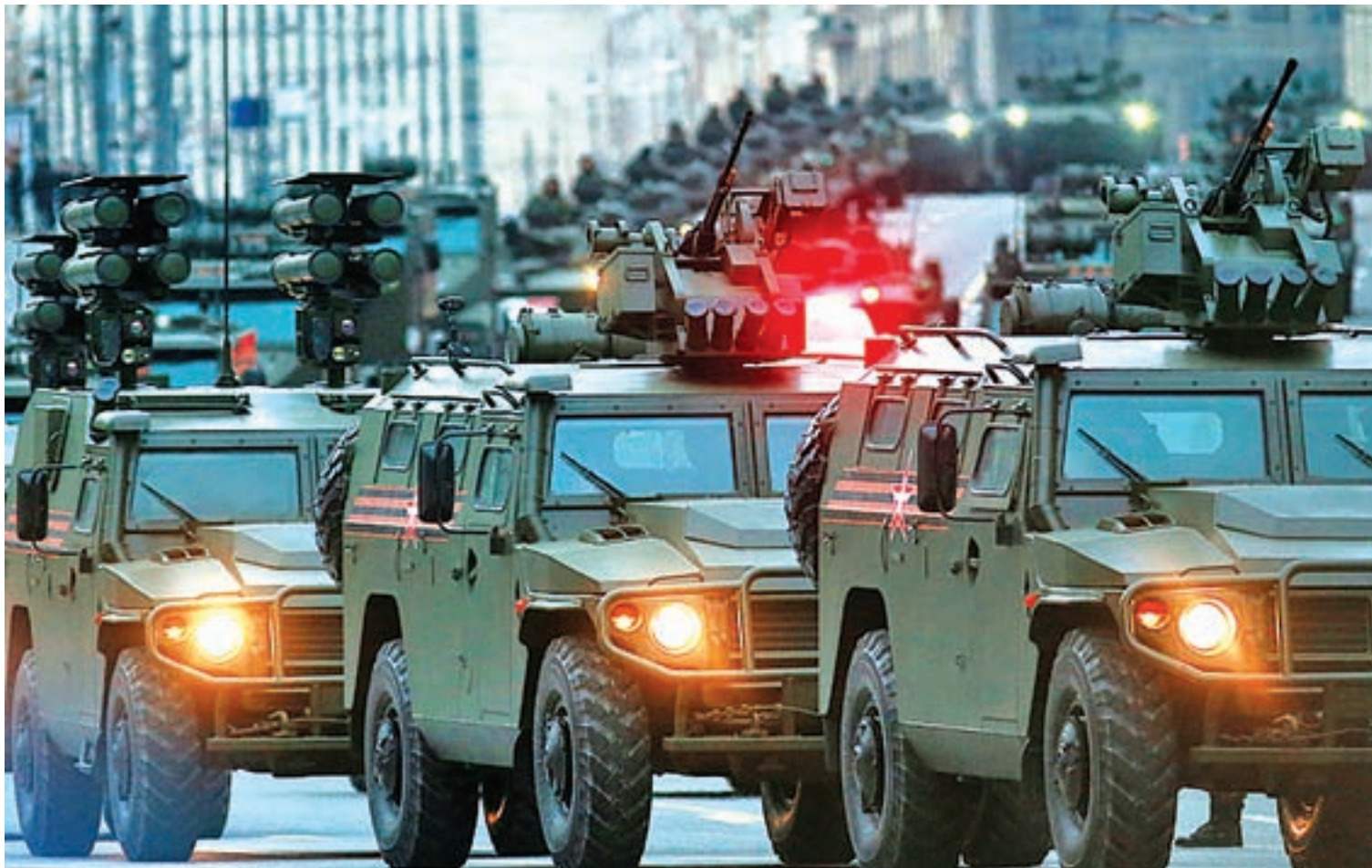
The vehicle can now move with no one inside and fire from a 30-mm cannon. PHOTO: TASS
