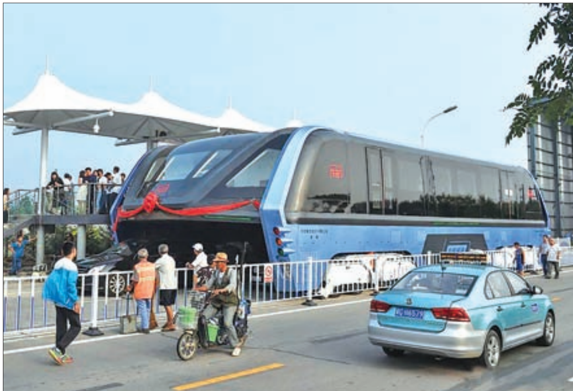
The transit elevated bus TEB-1 is on road test in Qinhuangdao, north China's Hebei Province, on 2 August, 2016. China's home-made transit elevated bus, TEB-1, conducted a road test running Tuesday. The 22-metre-long, 7.8-metre-wide and 4.8-metre-high TEB-1 can carry up to 300 passengers. The passenger compartment of this futuristic public bus rises far above other vehicles on the road, allowing cars to pass underneath. PHOTO: XINHUA
