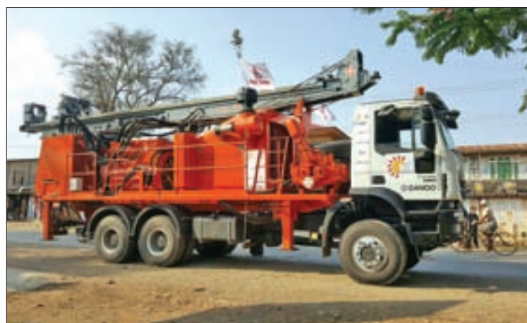
KBZ foundation's new machinery can drill down up to a depth of 1,800ft. PHOTO: KBZ
