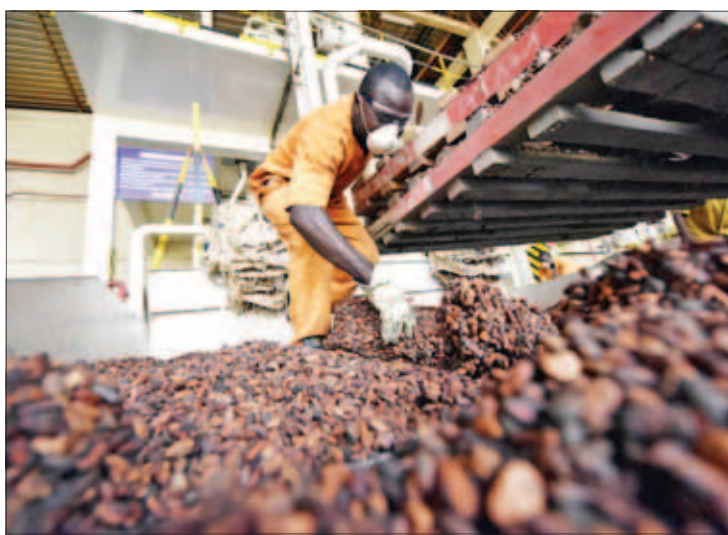
An employee of the CEMOI chocolate factory empties bags of cocoa beans onto a metal grate for the beans to be cleaned at the CEMOI cocoa processing plant in Abidjan on March 25. Photo: AFP
