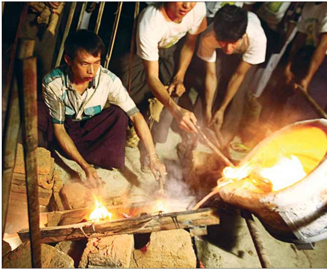
Volunteers pour molten bronze into the bell's mould inside a pit. Photo: Phyo Wai Kyaw
