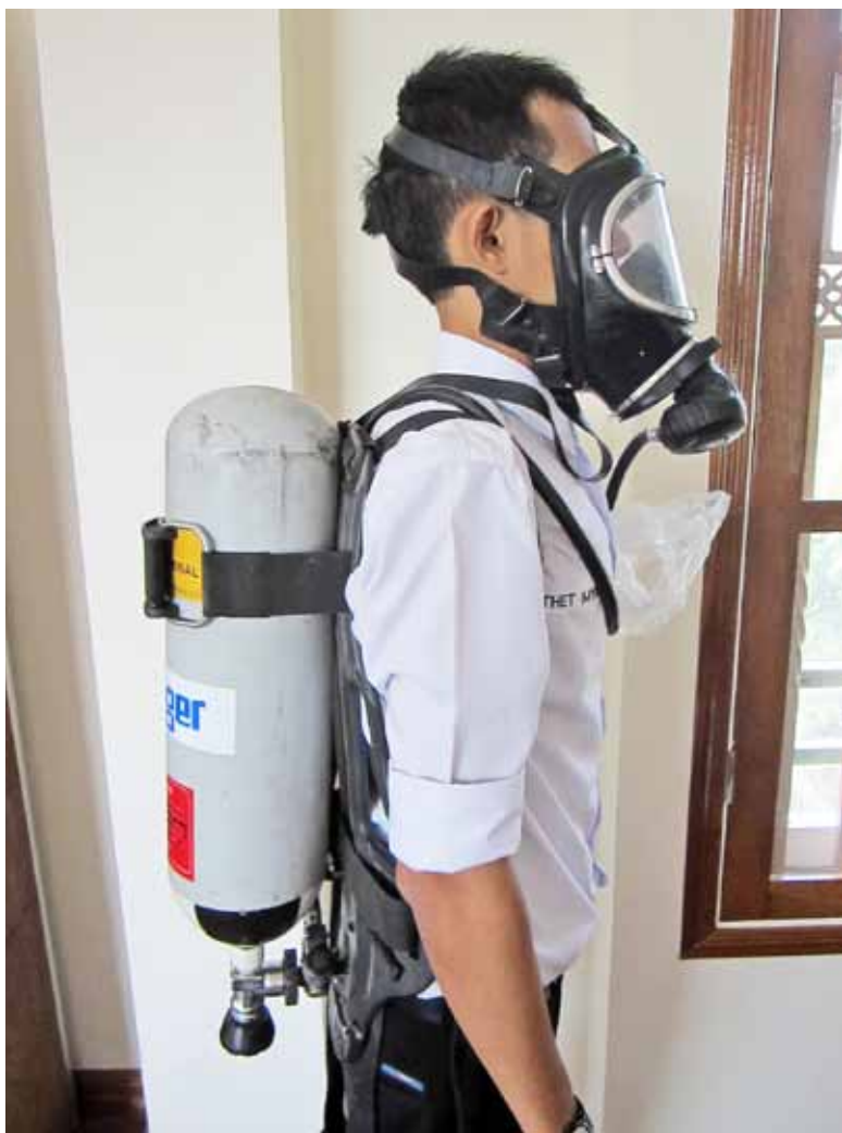
A breathing apparatus set is worn when entering the enclosed space of the cargo area. It prevents suffocation due to lack of oxygen and poisoning due to harmful chemicals. Photo: Jessica Mudditt
