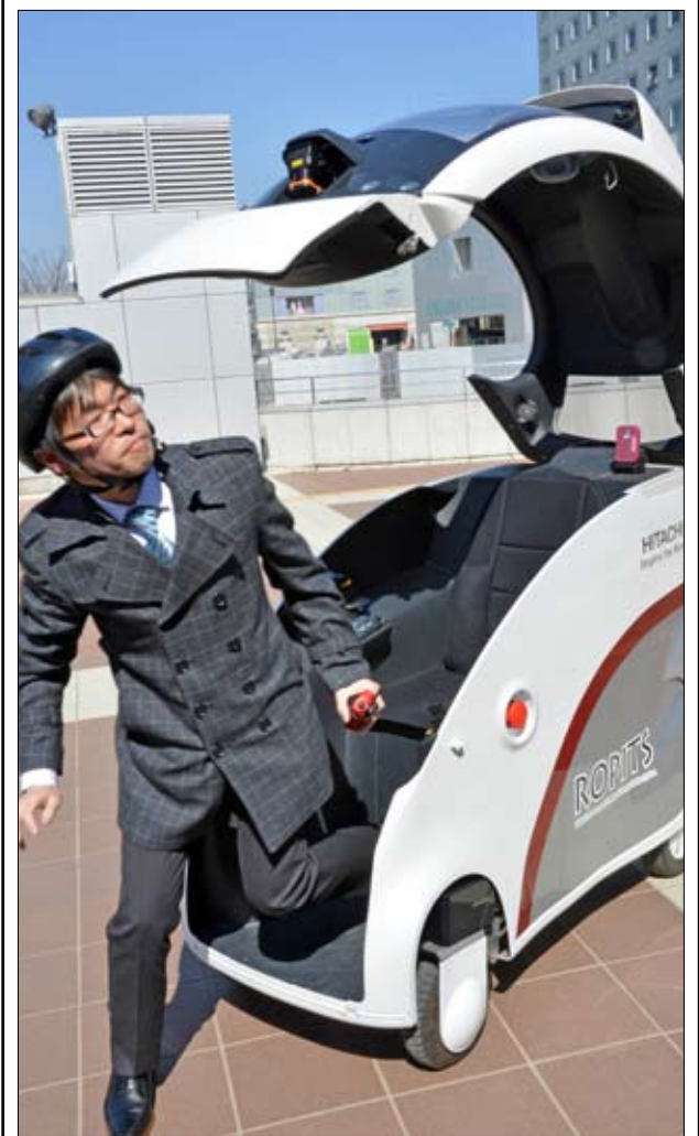
A Hitachi employee disembarks from a mobility robot unveiled at the Japanese high-tech maker’s facility at Tsukuba Science City in Japan on March 12. The single seat vehicle is known as Ropit, an abbreviation for Robot for Personal Intelligent Transport System. The vehicle, which is designed to travel on footpaths, can pick up and drop off passengers autonomously. It navigates using GPS and relies on cameras and 2D and 3D laser distance sensors to avoid pedestrians and other obstacles. It can also be controlled by a joystick controller in the cockpit. Ropit was designed for use by the elderly and those whose mobility is impaired. It is powered by a lithium ion battery and travels at speeds of up to six kilometres an hour (3.7mph). Pic: AFP
