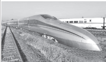
The six-car train with a fairshaped head is the newest in the CRH series. China's largest rail vehicle maker, CSR Corp Ltd, over the weekend launched its first test train that features speeds reaching up to 500 km per hour.— XINHUA
