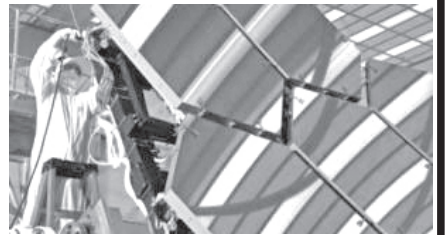
The James Webb Space Telescope mirrors have completed deep-freeze tests and are removed from the X-ray and Cryogenic test Facility at Marshall Space Flight Centre.—INTERNET
