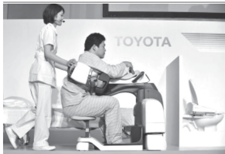
Fujita Health University senior assistant professor Yukari Suzuki (L) demonstrates a prototype robot 'Patient Transfer Assist' reducing the heavy physical burden of moving patients, developed by Japan's Toyota Motor Corporation, during a press preview at a showroom in Tokyo, on 1 November.—INTERNET
