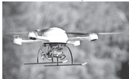
The Microdrone md4-200, a four-propeller "quadcopter" that weighs in at just 35 ounces.—INTERNET
