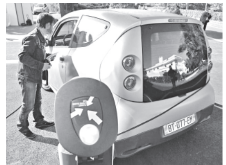
A member of the media takes a look at a Bluecar, an electric powered car made by French company Bolloré, at a media presentation in Vaucresson, west of Paris, Friday on 30 Sept, 2011. The Bluecars have a range of 250km, 155 miles, in urban use, a maximum speed of 130km/h, 80 miles per hour, and will be available in the streets of Paris under the name of Autolib. The four-seat Bluecars are to be positioned at 1,200 stations in metropolitan Paris and will be available around the clock. Users must have a valid driver's license and pay a subscription fee to borrow one of the vehicles. —INTERNET
