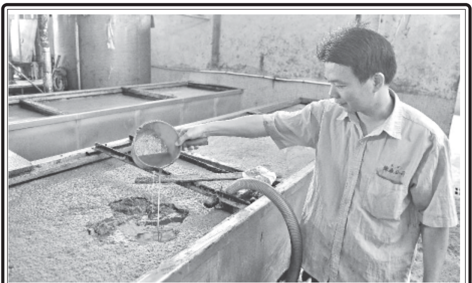
A worker separates oil from water at a kitchen waste disposal company called Lusen in Foshan, south China's Guangdong Province, 22 Sept, 2011. Kitchen gutter oil is collected and processed here to be refined as biodiesel. However, kitchen leftovers disposal companies such as Lusen are stranded due to less supply of the oil. According to Li Yaosong, president of Lusen, the daily reclaimed oil volume dropped from 20 tons in 2004 to 10 tons presently in the company, accounting for 20% in the whole reclaimed kitchen oil volume of the city's Nanhai District. Part of the rest sneaked back to dining tables through an underground muck-money network. Being in charge of the oil recycle business of Nanhai, Lusen signed contracts with 5,000 local restaurants, among which over 3,000 restaurants didn't supply their waste oil to the company because of low purchasing price provided.—XINHUA
