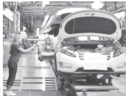
United Auto Workers union member Carrie Attwood uses an ergonomic arm to install a front seat in a Chevrolet Volt electric vehicle at General Motors Detroit-Hamtramck assembly plant in Hamtramck, Michigan on 27 July, 2011.
