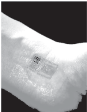
An ultrathin, electronic patch with the mechanics of skin, applied to the wrist for EMG and other measurements. Credit: University of Illinois, John Rogers.—INTERNET
