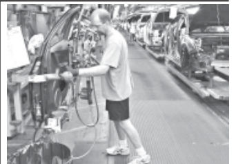
worker prepares to install a door on the new Chevrolet Cruze car as it moves along the assembly line at the General Motors Cruze assembly plant in Lordstown, Ohio on 22
