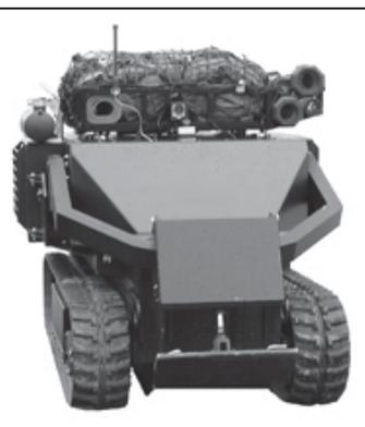
The bulldozer-size ACER robot can handle tasks like clearing explosives and hauling cargo.
