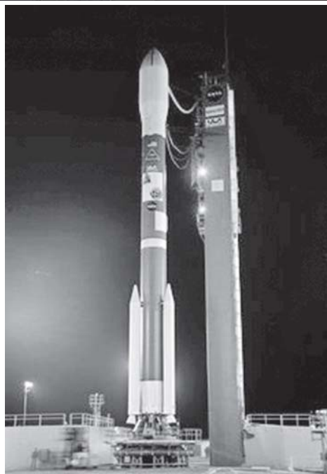
In this image provided by NASA the Delta II rocket with its Aquarius/SAC-D spacecraft payload is seen as the service structure is rolled back on 9 June, 2011, at Vandenberg Air Force Base, Calif.
