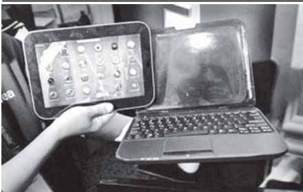
The Lenovo IdeaPad UI Hybrid device, which combines LePad, a 10-inch Android-powered tablet (L) with a Windows-powered base station.
