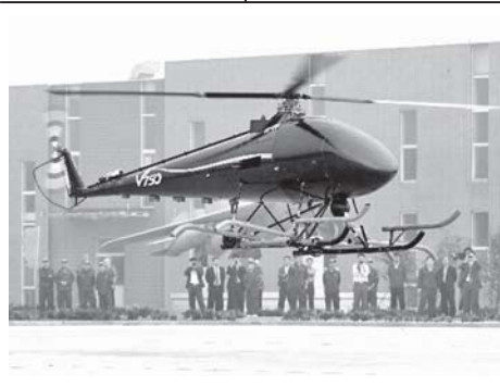
Photo taken on 7 May, 2011 shows the "V750" pilotless helicopter during a test flight in Weifang of east China's Shandong Province. The 757 kilogramme helicopter has a maximum load capacity of 80 kilogramme. XINHUA
