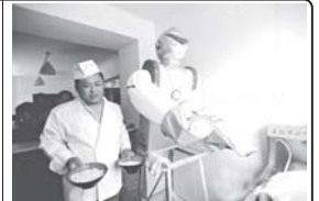
A robot chef slices noodles in a noodle restaurant in Shenyang, capital of northeast China's Liaoning Province, on 26 April, 2011. According to the boss's introduction, the robot took 20,000 yuan, and three times efficient than a chef, consuming only 1 kilowatt-hour in 10 hours.
