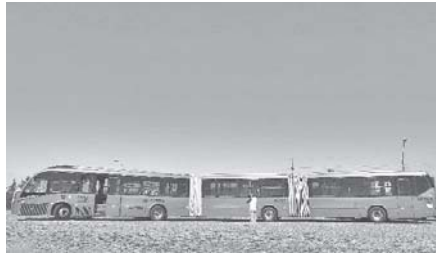
A view of what the Curitiba City Hall is calling the world's longest articulated bus, as it was presented to the press before going into service on the city's public transportation grid, in Curitiba. The bus, made in Brazil by Volvo with a Neobus chassis, has a capacity of 250 passengers, is 28 metres (92 ft) long, 2.6 metres (8.5 ft) wide, and powered with biodiesel made from soybeans.
