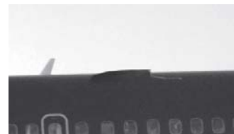
This photo provided by passenger Don Nelson, shows fuselage rupture that happened in-flight on a Southwest Airlines aircraft on 1 April, 2011.—INTERNET
