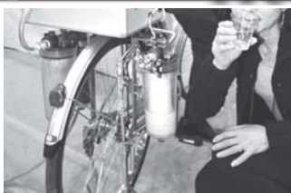
Japanese water purifier venture Nippon Basic displays a portable water purifying system “Cycloclean,” powered by pedaling a bicycle to make a maximum of 5 liter of clean water in a minute at a technology fair in Tokyo.—INTERNET
