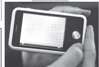
A new product from Ephone International Pte Ltd is displayed at the 3GSM World Congress in Barcelona, Spain. The EPI Life mobile phone comes complete with mini electrocardiogram and takes a user’s pulse when he or she presses their fingers on a receptor.
