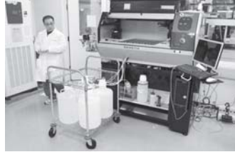
Staff scientist Marcus Jones walks towards the Genetex Qarray2 Micro Array Printer used for spotting DNA and protein in the laboratory at the J Craig Venter Institute in Rockville, Maryland, 29 March, 2010.—INTERNET
