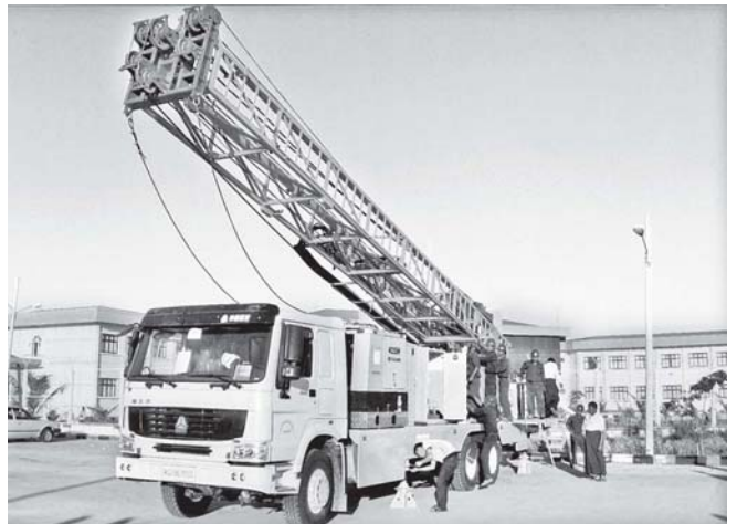
RG truck-mounted drilling rig manufactured by China seen in its preparatory work.
