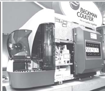
A Flow Cytometer which is used to identify stem cells based on light scatter and fluorescence is put on view at the Beckman Coulter exhibit during the 2010 World Stem Cell Summit at the Detroit Marriott Renaissance Centre 4 Oct, 2010 in Detroit, Michigan. More than 1,200 scientists and researchers from around the world are expected to attend the summit that focuses on the advancement of embryonic stem cell research.
