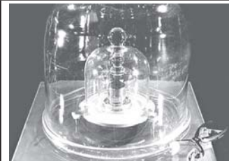
The original cylinder of platinum and iridium used as the standard weight for one kilogramme. Scientists said Monday they were moving closer to coming up with a non-physical definition of the kilo after discovering the metal artefact used as the international standard had shed a little weight.
