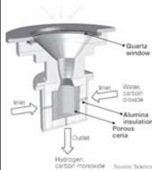
In the prototype, sunlight heats a ceria cylinder which breaks down water or carbon dioxide.— INTERNET
