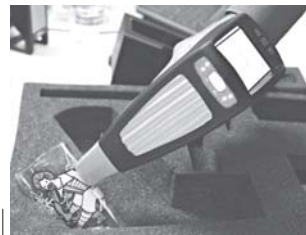
This on 9 Sept, 2010 photo shows an Olympus Innov-X Delta Handheld XRF Analyzer testing glassware decorated with a Ronald McDonald character for cadmium, lead and other toxic elements in Los Angeles. The device is used for the analysis of environmental, geological, biological, industrial and other samples.—INTERNET
