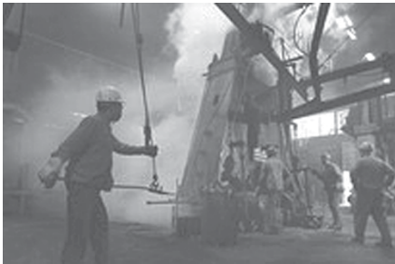
In this 18 Oct, 2010 photo, workers get ready to pull a piece of forged steel to be used in a heavy load helicopter out of a giant press at SifCo Ind.—INTERNET
