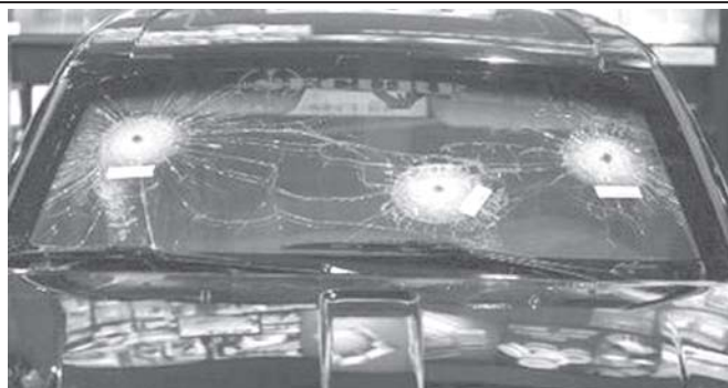
Impacts of bullets are seen on a piece of bullet-proof glass during a security exhibition in Mexico City, on 21 April, 2010. The exhibition presents the latest in police, civil defence security equipment.—XINHUA
