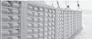
A view of the hull of the Plastiki, a 60-foot catamaran made mostly from recycled plastic in San Francisco Bay.
