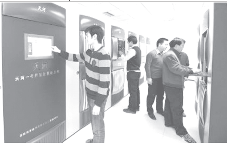
Technician tests Tianhe-1 (TH-1) supercomputer at north China's Tianjin, on 25 Dec, 2009. The supercomputer, named Tianhe, meaning Milky Way, is theoretically able to do more than 1 quadrillion calculations per second at peak speed, which was already partly installed in Tianjin.—XINHUA
