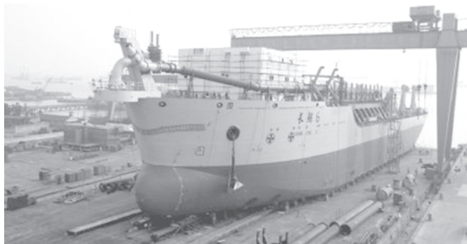
Chang Jing 6, one of the country's largest trailing suction hopper dredger, is to be launched in Nantong, east China's Jiangsu Province, on 3 Dec, 2009. With a cabin space of 13,280 cubic metres, the dredger of Changjing 6, with China's proprietary intellectual property rights, will be earmarked for dredging and hydraulic filling on the coastal ports and Yangtze River's navigational routes, in addition to coastal maintenance projects.—XINHUA
