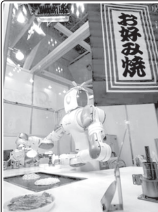
“Okonomiyaki Robot” demonstrates its ability to cook Japanese traditional food Okonomiyaki, a savoury pancake, during the international robot exhibition 2009 in Tokyo on 25 Nov, 2009. The robot which has 15 joints, can take verbal orders from customers and use standard kitchen utensils. The banner reads, “Okonomiyaki”.
