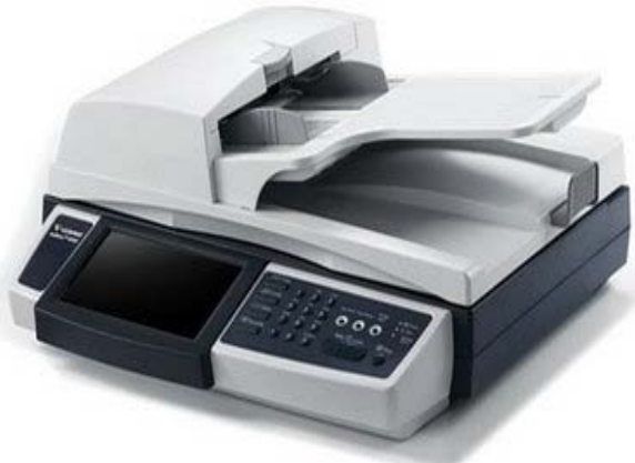
The Visioneer NetScan 4000 is a new duplex color network scanner with LCD touch screen that scans documents at 20 ppm or 14 ipm in duplex. It supports LDAP for direct access to Microsoft Exchange Server email directories and SMTP server support.—INTERNET
