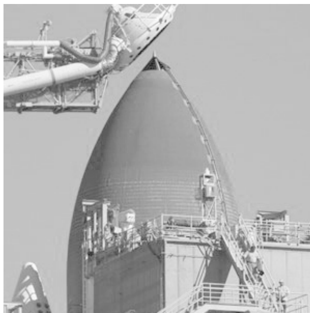
Two workers walk away after inspecting the top of the external tank on the space shuttle Atlantis at the Kennedy Space Center in Cape Canaveral, Fla. INTERENT
