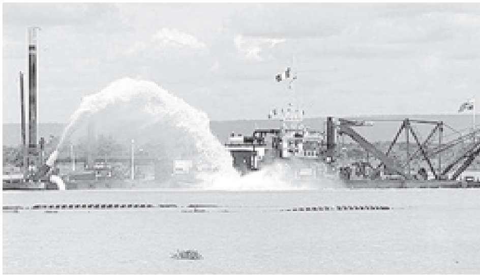
A dredger flushing water from the River Niger in Lokoja in the Kogi State, to boost navigation and commerce along a 572 kilometres stretch of the river. After decades of delay and wrangling by resisting riverine communities, Nigeria has launched a multi-million-dollar dredging exercise to boost navigation and commerce on the Niger River.
