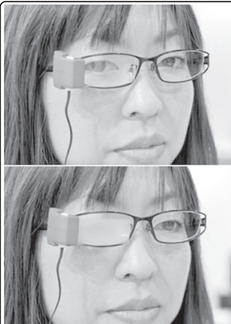
A Japanese eyewear maker Masunaga Optical employee displays the blinking "Wink Glasses", which are supposed to help prevent dry-eye when the users concentrate on video gaming or on the Internet.
